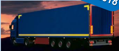
Retro-Reflective Installation (UN R104)
