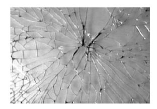
Fig. 3: Safety glass after broken
