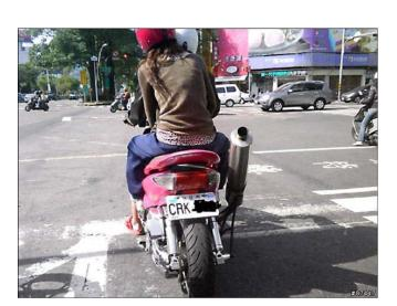
**Background:** Due to the angle of tailpipe is too large, the exhaust gas could blow to other moped/motorcycle rider.
