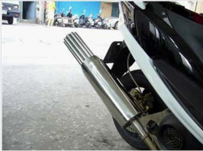
**Background:** Due to the angle of tailpipe is too large, the exhaust gas could blow to other moped/motorcycle rider.
